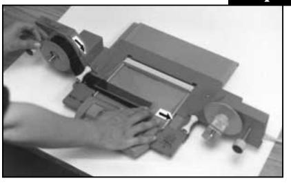
LOAD FILM ON LEFT SPINDLE: Feed film from over the top of reel.
